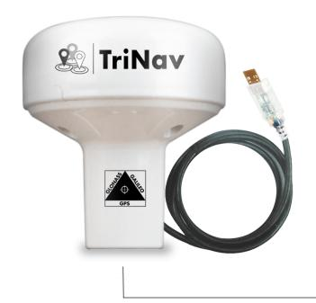
The GPS160USB variant ships with a 5m cable. It's self powered from the USB source (PC, MAC or Linux). When installed, a virtual COM port is created on the host PC so navigation programs can receive positioning data.
