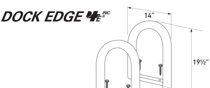
DockEdge+ welded aluminum ladder dimensions for Part #s 2013-F, 2014-F & 2015-F
