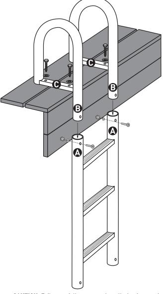
CAUTION: Failure to follow proper installation instructions may lead to product failure and personal injury. Ladder must be mounted flush with the dock face board. Regularly inspect for wear or damage. Replace as necessary. (DO NOT EXCEED THE LADDERS' MAXIMUM CAPACITY OF 665LB. (302KG))
