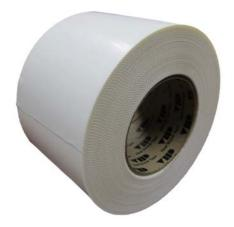
Heat shrink tape is a polyethylene backed tape with very good adhesion which is used for repairing holes in poly film, taping on zipper access doors, and taping pleats on the shrink wrap. The light-duty heat shrink tape is a low-cost alternative to our standard heat shrink tape and works in the same manner. \*Does not contain UV Inhibitors\*
