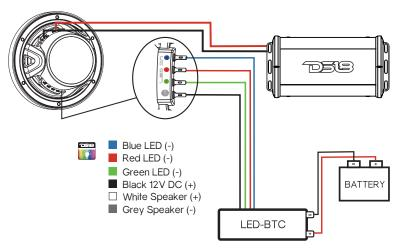
To connect without LED Control Module (LED-BTC), Connect as Shown in the Following Diagram;
