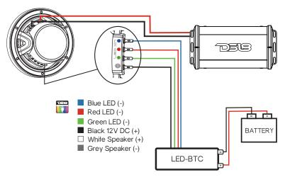
To connect without LED Control Module (LED-BTC), Connect as Shown in the Following Diagram;
