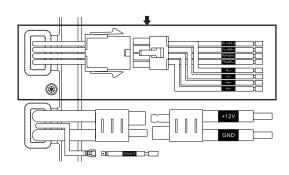
and insert them into the block terminal while being careful that there is no loose or frayed strands of wire and tighten the Allen head screw down on the terminal till the wire is tightly secured in place. If the wires ever come in contact with each other the amplifier will go into protection.
