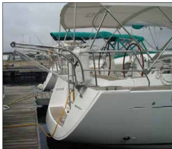
2007 Beneteau 49 with Custom Davit Mounting Brackets
