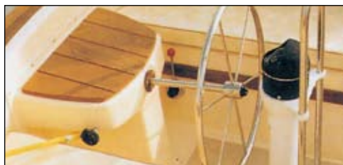
The Island Packet above shows a typical installation of the Edson #317 Compass Pedestal.
