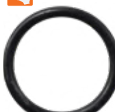
25-00153-1 O-Ring Mercury/Mariner 2-cyl, 4 Hp | 4-cyl, 75-150 Hp outboards. ID: 0.4375" | OD: 0.5625" | W: 0.0625" Xref: Mercury 62706 SIE: 18-7102-9
