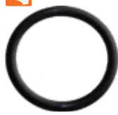
25-00157-1 O-Ring Mercury/Mariner 2-cyl, 40 Hp | 3-cyl, 65-70 Hp | 4-cylinder, 75-85 Hp | 6-cyl, 90-115 Hp | V6, 135-300 Hp outboards. ID: 1.25" | OD: 1.4375" | W: 0.0937" Xref: Mercury 35480 SIE: 18-7411-9
