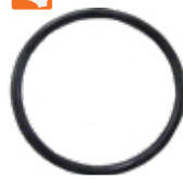
25-00207 O-Ring Mercury/Mariner 2-cyl, 6-25 Hp | 4-cyl, 65-120 | 6-cyl, 90-150 Hp | V6, 150-225 Hp outboards. ID: 2.0" | OD: 2.25" | W: 0.125" Xref: Mercury 33145 SIE: 18-7162
