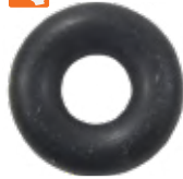
25-00165-1 O-Ring Mercury/Mariner 2-cyl, 8-40 Hp | 3-Cyl, 30-40 Hp | 4-cyl, 40 Hp outboards. ID: 0.242" | OD: 0.570" | W: 0.164" Xref: Mercury 85594 SIE: 18-7100-9
