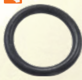
25-00209-1 O-Ring Mercury/Mariner 2-cyl, 35 Hp | 3-cyl, 50-90 Hp | 4-cyl, 45-200 Hp | 6-cyl, 90-115 | V6, 135-300 Hp outboards. ID: 0.625" | OD: 0.8125" | W: 0.0937" Xref: Mercury 45711 SIE: 18-7174-9
