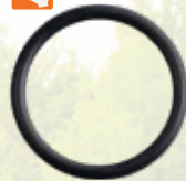
25-00208-1 O-Ring Mercury/Mariner 3-cyl, 65-90 Hp | 4-cyl, 90-200 Hp | V6, 135-300 Hp outboards. ID: 1.375" | OD: 1.625" | W: 0.125" Xref: Mercury 33504 SIE: 18-7170-9
