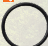
25-00162-1 O-Ring Mark & Mercury/Mariner 1-cyl, 3.9-4.5 Hp | 2-cyl, 6-20 Hp outboards. ID: 0.4375" | OD: 0.625" | W: 0.09375" Xref: Mercury 26802 SIE: 18-7180-9
