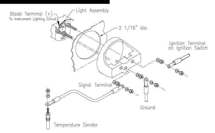
**CAUTION:** Disconnect the battery during installation. Tighten nuts on the backclamp only slightly more than you can tighten with your fingers. Six inch-pounds of torque is sufficient. Overtightening could result in damage to the instrument and may void your warranty.
