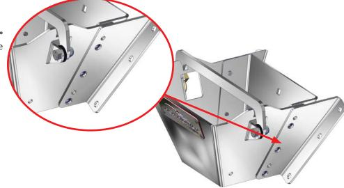
**3.** Install using (2) ¼" Cap Screw and (2) Nylock Nuts per side.
