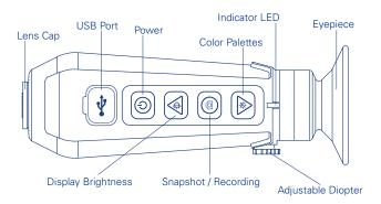
**Charging the OCEAN SCOUT-TK** – Use the included USB Cable and connect to a power source. The Indicator LED flashes while charging and blinks green when fully charged.
