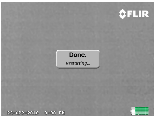
Notification screen of a successful load and pending restart to finish software update
