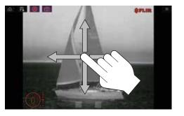
On a touchscreen MFD you can pan, tilt, and zoom the thermal camera image using the touchscreen:
