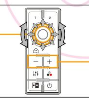
Use the circular Uni-controller to: Tilt the camera up and down, or pan it left and right (M200 Series only): press the inner-ring up, down, left, or right.
