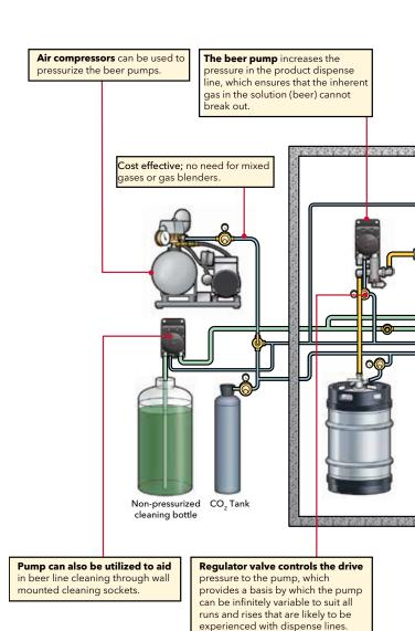
Flojet's BeerJet pumps are capable of pumping beer up to 240 meters horizontal or 30 meters vertical through a single line. The pump can dispense up to five taps from a single keg and has a service life of more than 250,000 liters.
