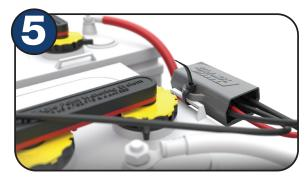
Secure the control box with a zip tie provided in a secure location.
