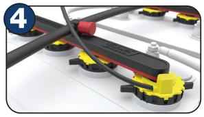
Lock each valve in place and reconnect the tubing.
