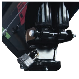
Lockable BULLDOG® coupler for added security
