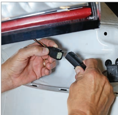
4. Plug the tail light into the T-One® connector.
