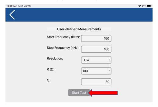
Press "Start Test" to run the test. You should get indications of "Calibrating" at the bottom of the screen and finally "Measuring". The whole process will take several moments. When finished you should have a curve something like the below.
