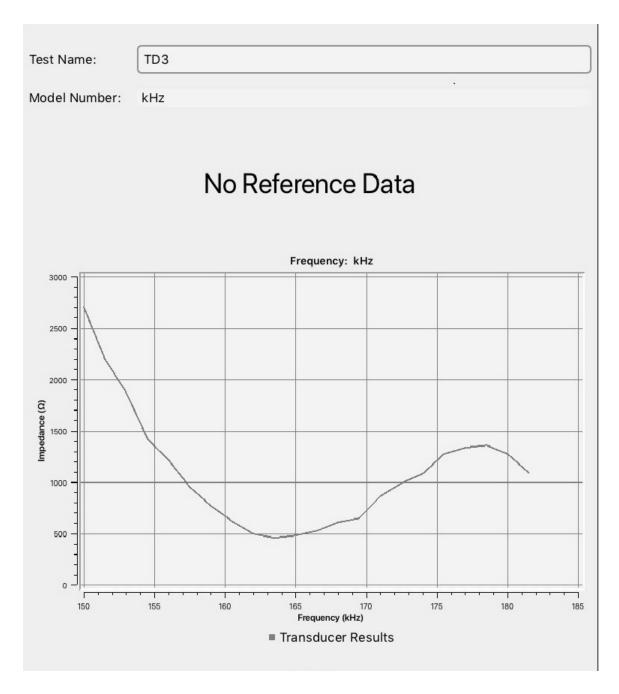
Repeat this procedure for each element by swapping in the next associated wire into **POSITION 11** of the breakout box. All elements should be close to the same curve shape. Please note that these readings were taken with the transducer placed on the Airmar Transducer Testing Block
