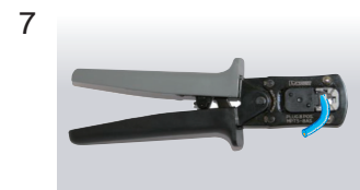
7 Using special crimping tool MPT5-8AS (PANDUIT CORP.), crimp the modular plug. Finally check the plug visually.
