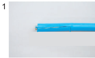
Expose inner vinyl sheath.
