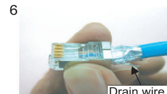
Insert the cable into the modular plug so that the folded part of the shield enters into the plug housing. The drain wire should be located on the tab side of the jack.
