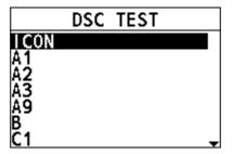
Step 3Press the Menu/DSC control to send the DSC test call.<br/>Your radio waits for an acknowledgement from the radio you called.
