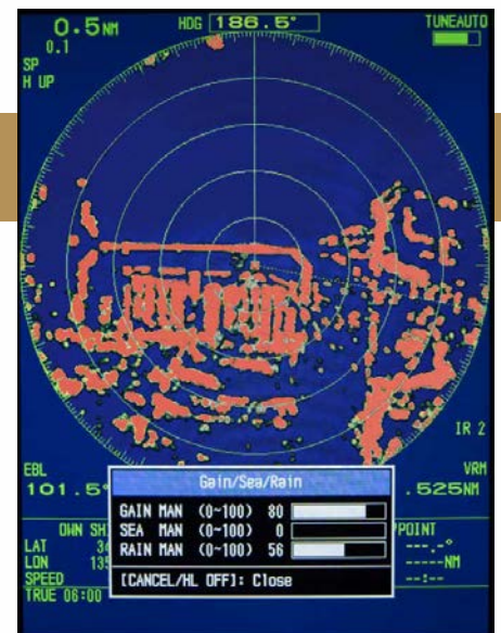
A/C Rain turned on, the marina appears clearly.
