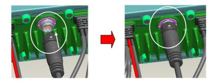
**Step 3** Secure the other end of the extension cable to the panel.
