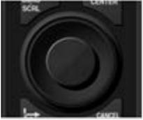
The large rotary knob offers a friendly operation for zoom in/out similar to the RotoKey™ of TZT9/14/BB. The big joystick makes it easier to move the cursor. With the TZTL12F/15F v3.01, pushing the joystick selects the highlighted items in contextual menus, settings, Layer, etc.
