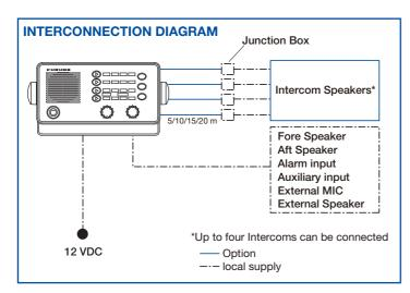
The LH-3000 can also function as an intercom, when connected to optional intercom speakers. Up to four intercoms can be connected for two-way communication between the bridge and one or all intercom stations.
