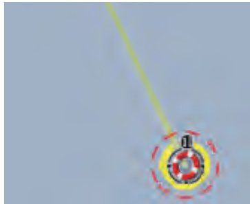
MOB mark on the chart plotter display
