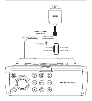
FUSION recommends that the MS-BT100 is mounted in an elevated position as far away from metal work as possible. This will ensure maximum range for Bluetooth audio streaming. Any barrier between the MS-BT100 and your streaming device will reduce the range.
