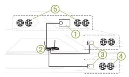
In the image above, one Apollo RA770 stereo ① connects to a wireless router ② and to two Apollo SRX400 zone stereos ③. The two FUSION PartyBus stereo zone stereos can stream sources from the FUSION PartyBus stereo.
