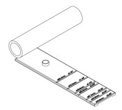
The raised, cable pass-through hole on the liner should fit into the cable pass-through hole on the waketower pipe.
