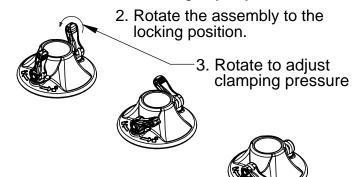
4. Push down on clamp to lock, lift up on clamp to open.
