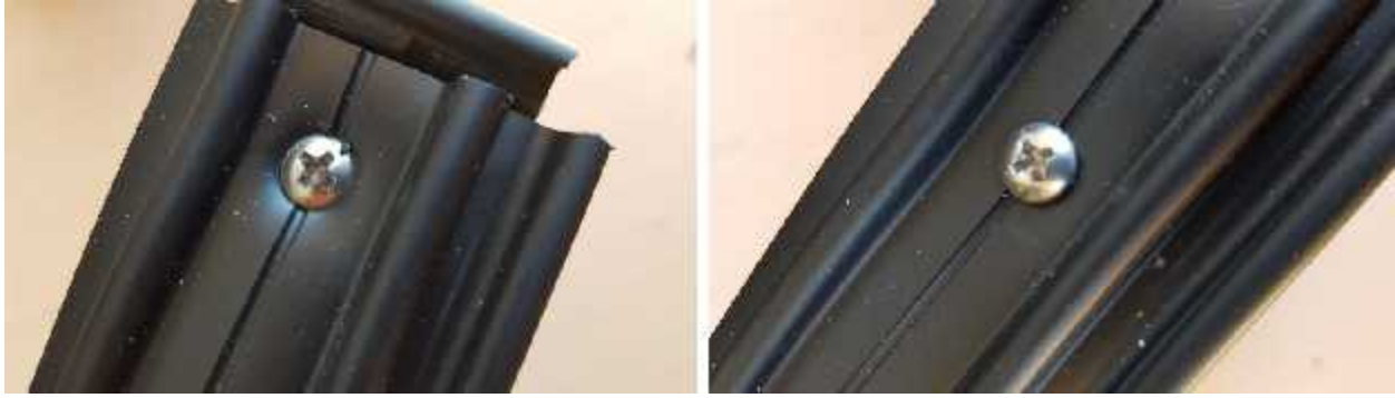
FIG 3.1 The screw on the left has been installed too tightly. The screw on the right has been installed correctly and just begins to bind the Bunk material.
