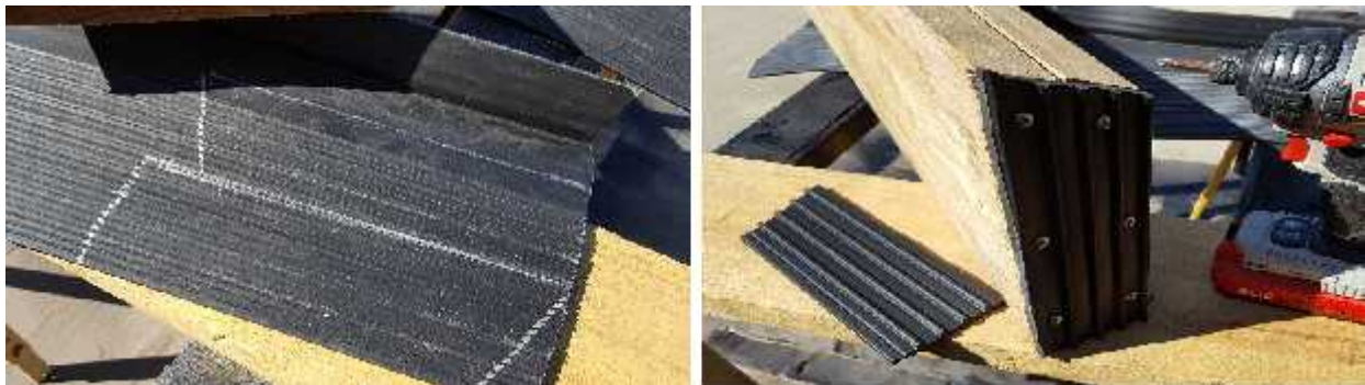
FIG 4.1 Use the end of the bunk Beam to create the pattern that you need for your end cap, once mounted trim the End of the cover or cap to complete the fit.
