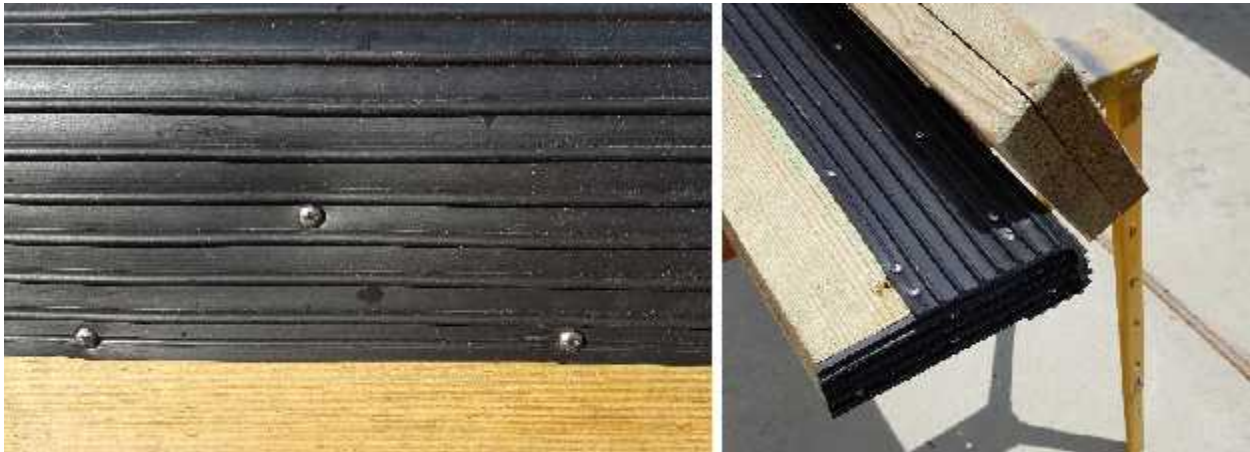
FIG 3.2 Additional screws installed to secure excess cover width. If desired cover can be trimmed to any final width. Ensure all screws are mounted within the channels and away from any facing that contacts the hull. Stainless Steel Staples can be used as well (not shown) as the primary mounting is done with the recommended screws.
