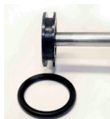
3. Remove the O-ring from the piston with a blunt tool. Do not damage the O-ring or the piston. Clean the O-ring and the piston recess.
