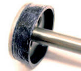
4. Apply a layer of new lubricant to the outer surface of the piston.
