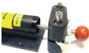
5. Carefully insert the piston rod and refit the bracket.
