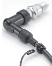
2 stroke install: Wrap pickup wire around spark plug lead.
