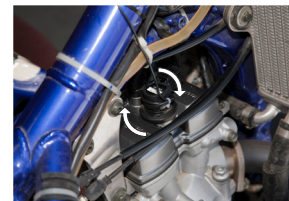
4 stroke installation: Wrap pickup wire around head of coil
