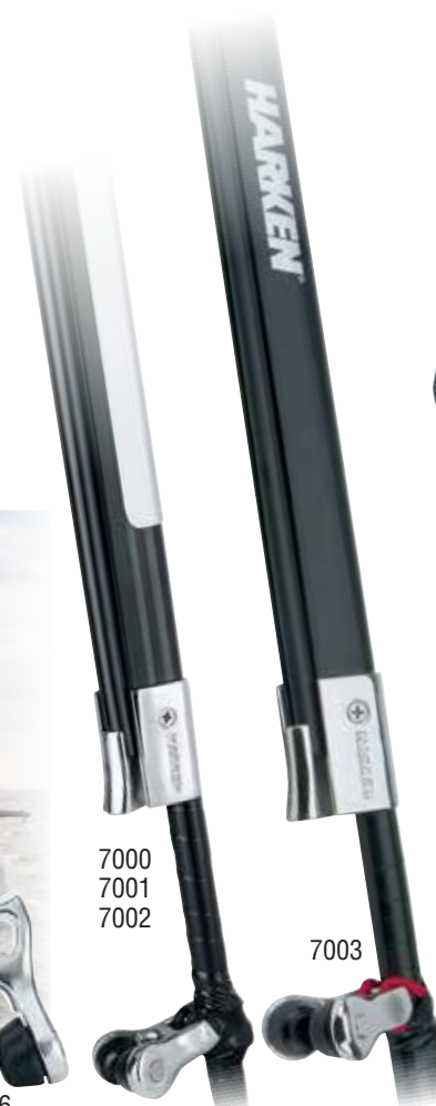
Feeder for smooth hoists: Funnel-shaped stainless feeder smoothly guides boltrope into headfoil for fast hoists.
