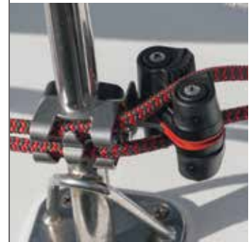
Outboard leads allow furling line to travel outboard of the stanchion to keep the sidedeck clear.
