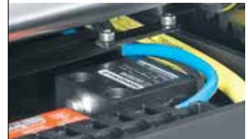
Two inner magnetic switches factory-set at the feeder's stroke limits prevent overtravel. Two outer fail-safe limit switches automatically engage the brake.
