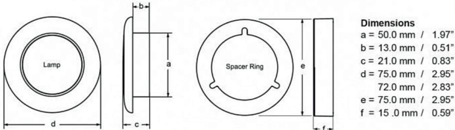
a = 50.0 mm / 1.97" b = 13.0 mm / 0.51" c = 21.0 mm / 0.83" d = 75.0 mm / 2.95" with plastic rim 72.0 mm / 2.83" with stainless steel rim e = 75.0 mm / 2.95"
