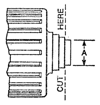
When cable diameter is greater than ring diameters "A"—cut off flush with next larger diameter rings.
