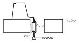
**NOTE**: The transducer must be submerged in water for reliable transducer detection. The bottom of the transducer should be even with the bottom of the ice or hang slightly below the bottom of the ice.
