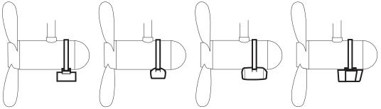
The transducer should be mounted forward of the motor shaft. Styles of transducer may differ from the illustration.
