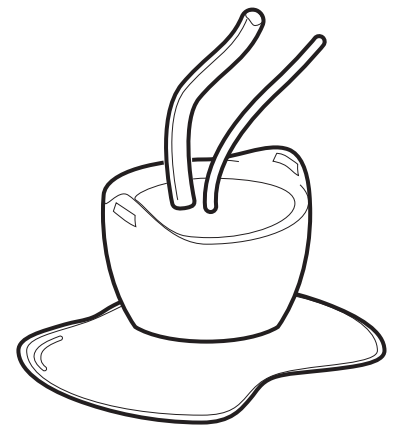
In-Hull Transducer with External Temperature Probe
