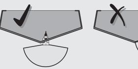
not interfere with the Side Imaging beams.
