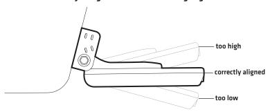
3. Hand tighten the two pivot bolts, using a 1/2" [13 mm] wrench.
