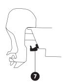
**Unobstructed View:** This jack plate installation gives the transducer safe distance from the motor and turbulence. The Side Imaging has a clear view side-to-side.
