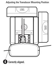
**Downward Slant:** The transducer has a natural downward slant of 4 to 5 degrees from leading edge to trailing edge. Looking at the back of the transducer, the seam should be slightly below the bottom of the hull.
