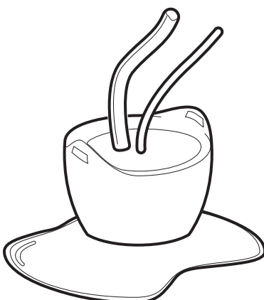
In-Hull Transducer with External Temperature Probe
