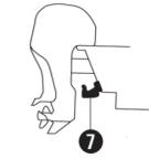
**Unobstructed View:** This jack plate installation gives the transducer safe distance from the motor and turbulence. The Side Imaging has a clear view side-to-side.
