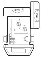
2. **Adjust the angle of the transducer,** so it is parallel with the length of the boat hull, with a slight down angle (approximately 5 degrees)
