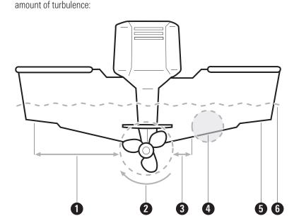
**1** Avoid areas where there is turbulent water flow. Turbulent water is normally confined to areas immediately aft of ribs, strakes, or rivets on the bottom of the boat, and in the immediate area of the propeller(s). The best way to locate turbulence-free water is to view the transom while the boat is
