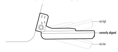
3. Hand tighten the two pivot bolts, using a 1/2" (13 mm) wrench.
