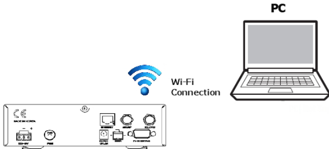
Figure 26 : ACU to PC Wifi Connection
