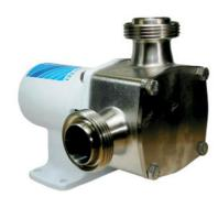
Jabsco Flexible Impeller Pumps are compact, easy to use and maintain. They handle low and high-viscosity liquids, gels and pastes and can pass suspended soft and hard solids. The smooth pulsation-free flow and gentle pumping action will not break down shear-sensitive or fragile liquids.
