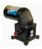
Multiple diaphragm PAR-MAX pumps from JABSCO are compact, quiet and durable. Self-priming is rapid, the bilge can be pumped virtually dry, and the pump is not harmed by dry running. Discharge heads should not exceed 3-4 metres for any of these pumps. They are supplied with an inlet strainer to keep out solids big enough to interfere with the pump's valves.
