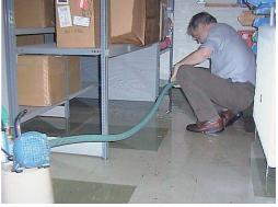
the pump can continue running for a while without damage after the liquid supply has run out. The larger Utility Pump models can safely run dry for as long as half an hour, thanks to an ingenious design of pump head that retains liquid while still pumping air.
