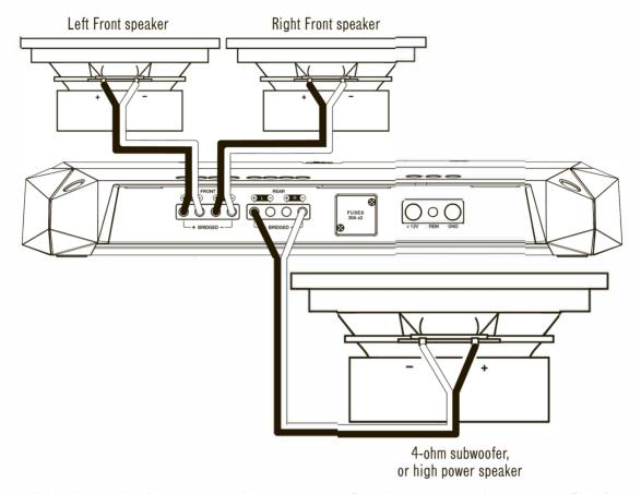
• 2-channel (bridged) operation: Connect one speaker's + lead to the Front L+ terminal, and the - lead to the Front R- terminal. Connect the other speaker's + lead to the Rear L+ terminal, and the - lead to the Rear R- terminal.
