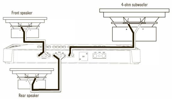
**NOTE:** Minimum speaker impedance for stereo full-range and subwoofer operation is 20hms. Minimum speaker impedance for bridged operation is 40hms.
