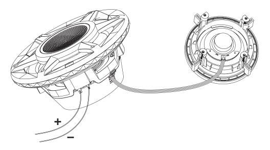
Place the tweeter in the mounting location, then turn each setscrew clockwise to tighten mounting brackets. Use caution so as not to overtighten. Snap the included outer ring over the mounting bracket to hide the setscrews.
