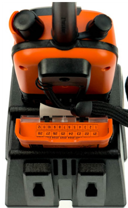
Figure 5 Radio in the charging bay and GM-DSS battery in the storage bay
